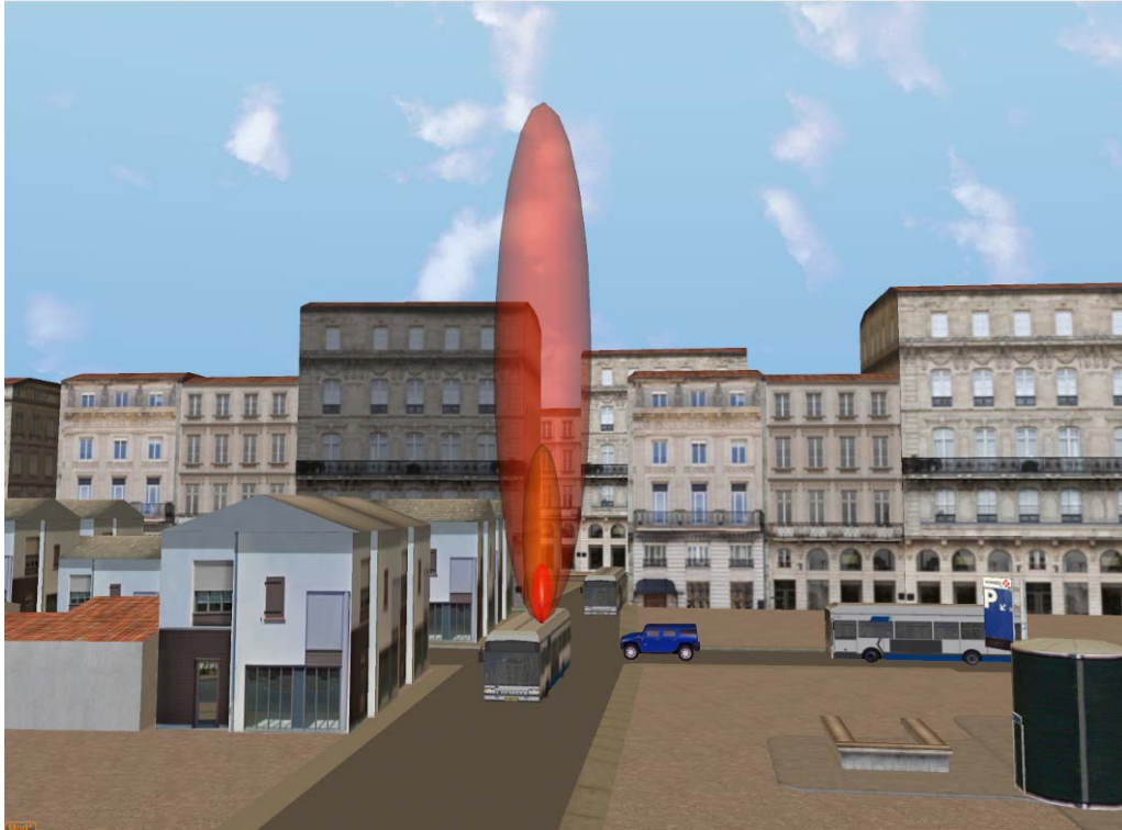
Figure 1 Example of the three transparent colours to show different hydrogen concentrations in virtual reality by CRISE
